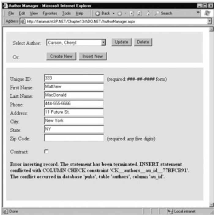
Figure 13-9: A failed insertion
