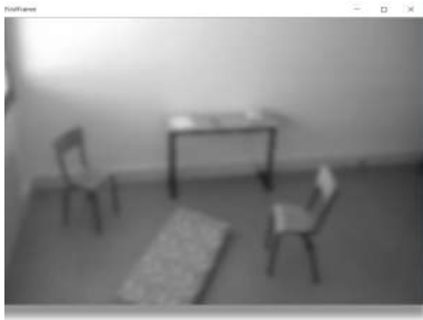
Fig. 2. First frame which will be compared with all other frames and the areas changing will be represented as contours.
