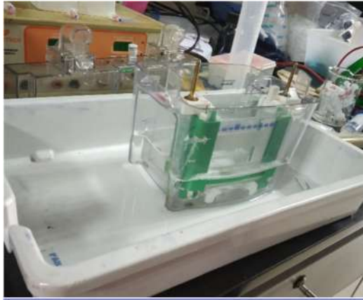
Fig. 3. Buffer tank with gel loaded with samples
