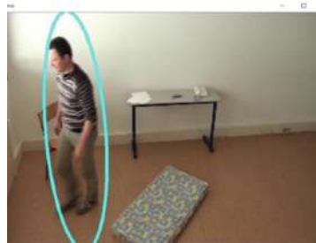
Fig. 5. Marking area of interest with bounding ellipse and determining angle and size of ellipse. Then using Eq. (1) to determine it is a fall or not.
