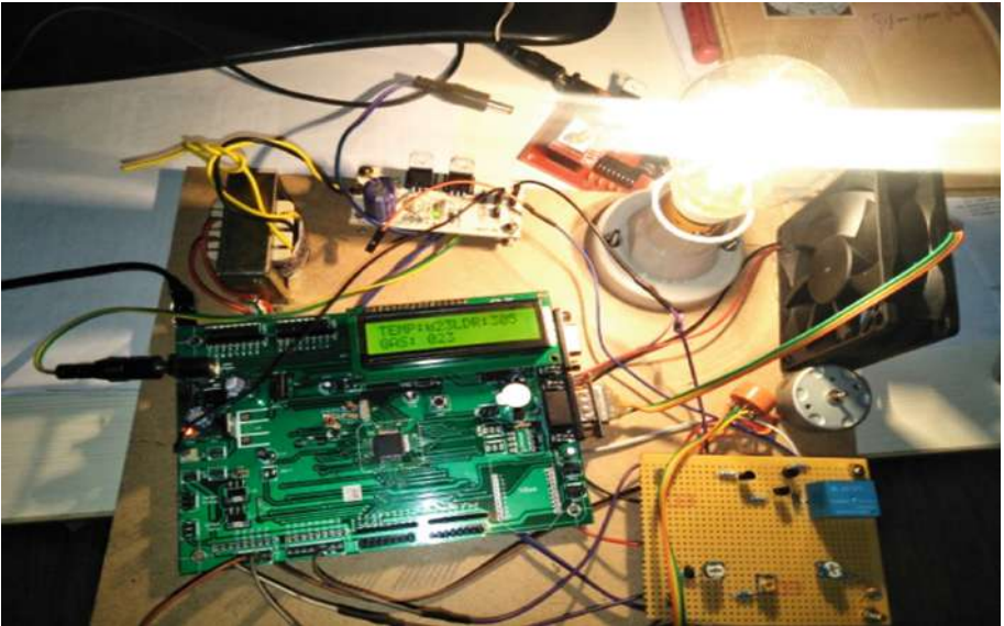
Fig. 5. The LDR value is below threshold value so that Bulb will turn ON
