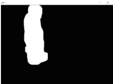
Fig. 4. Silhouette of the moving body of human. This was done by thresholding. For finer tuning, dilation was added by image processing technique.
