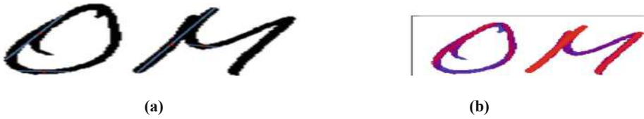
Fig. 4. (a) Longest traversing segment for 4 different pixels, (b) Length of maximum traversing segment: red corresponds to the maximum length and blue to the minimum one.
