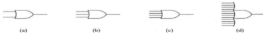
Fig. 2.6 OR gate symbols: (a) Two-input, (b) Three-input, (c) Four input, (d) Twelve-input
