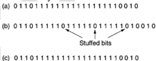
Fig: Bit stuffing. A) The original data. B) The data as they appear on the line. c) The data as they are stored in the receiver's memory after destuffing.
