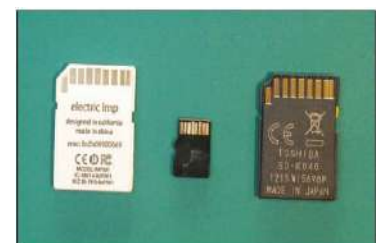
The rear of (from left to right): an Electric Imp, a micro SD card, an SD card.
