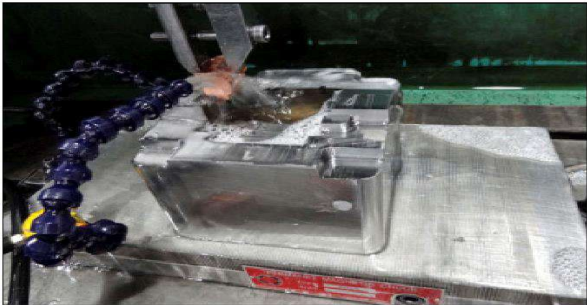
One of the moulds for BERG's Little Printer being finished on an EDM machine.
