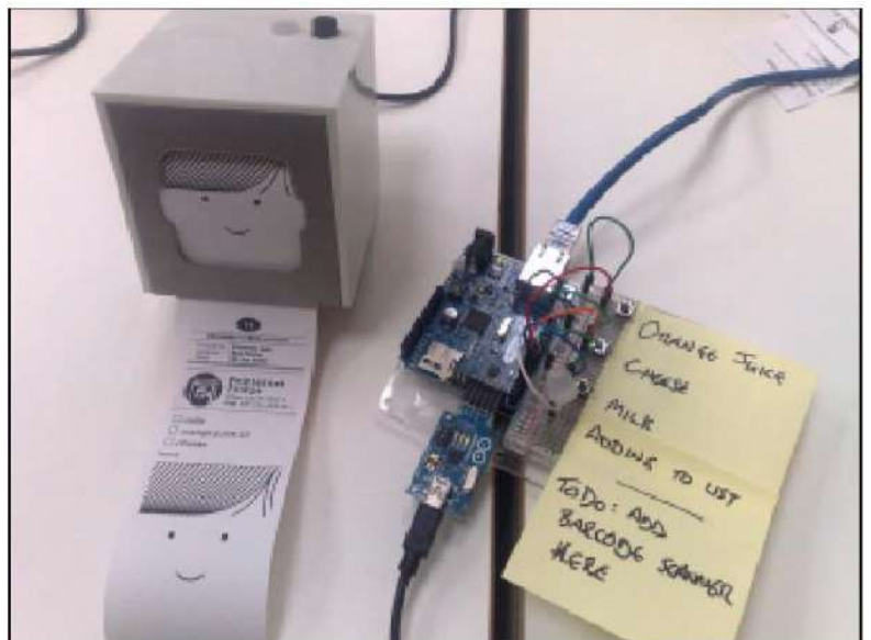
The finished prototype of the Printernet Fridge.
