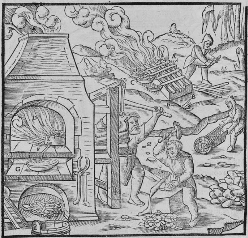
Figure 4.3 Smelting bismuth ore using pulverized charcoal, from Georgius Agricola, De re metallica (Basel: 1556). Reproduced with permission of the University of Delaware, Special Collections, Newark, Delaware.
